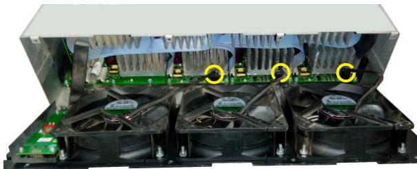
Figure 3: Disconnect the fan wires
